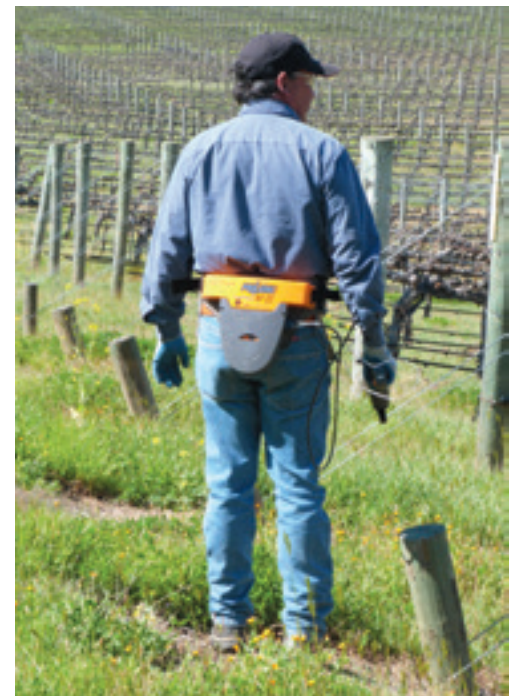
Portable battery packs for electric hand-held shears and tying guns
